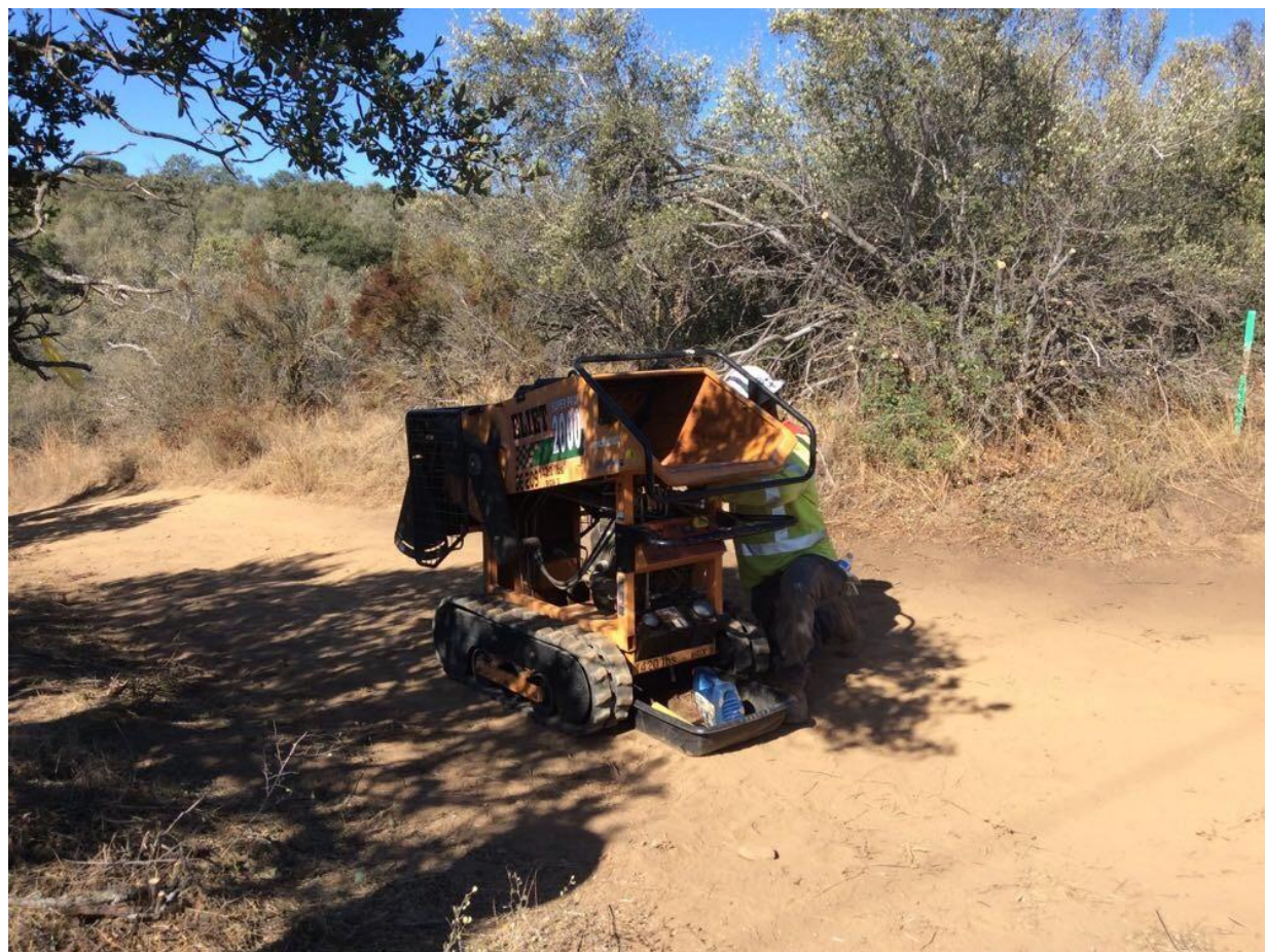
Photo 4: While a worker conducted equipment maintenance on a chipping machine at Pole Z273032 (TL 625C), a drip pan was placed beneath the machine to prevent potential leaks or spills from being discharged into the soil in accordance with the Spill Response and Notification Plan and MM PHS-2.
